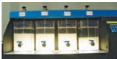
Four weeks of jar testing determined media capacity, effective elution of fluoride, arsenic and sludge and wastewater quality for disposal to the WWTP.
