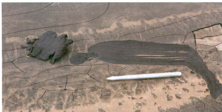
THIS IS A CLOSE-UP OF IRON AND MANGANESE SLUDGE AFTER DEWATERING. ONCE SUFFICIENTLY DRY, THE IRON AND MANGANESE SLUDGE IS REMOVED BY TRUCK FOR PROPER DISPOSAL.
